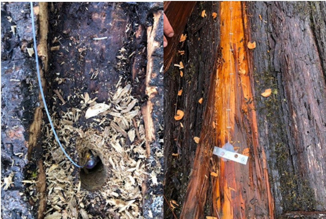
Figure 4.7-2. Large Wood installation of radiotags. Hole drilled and radiotag inserted (left). Hole filled with waterproof adhesive and metal brace screwed on top of hole and antenna stapled to log surface where bark was removed (right).
