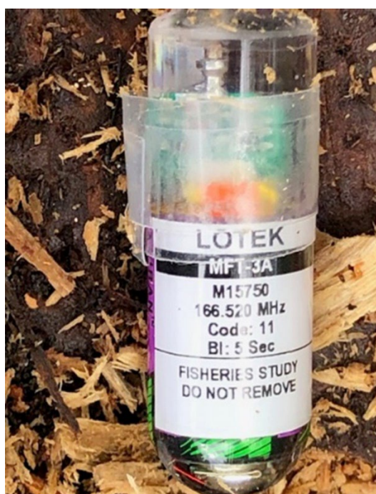
Figure 4.7-1. Lotek MFT-3A radiotag used to track large wood.
