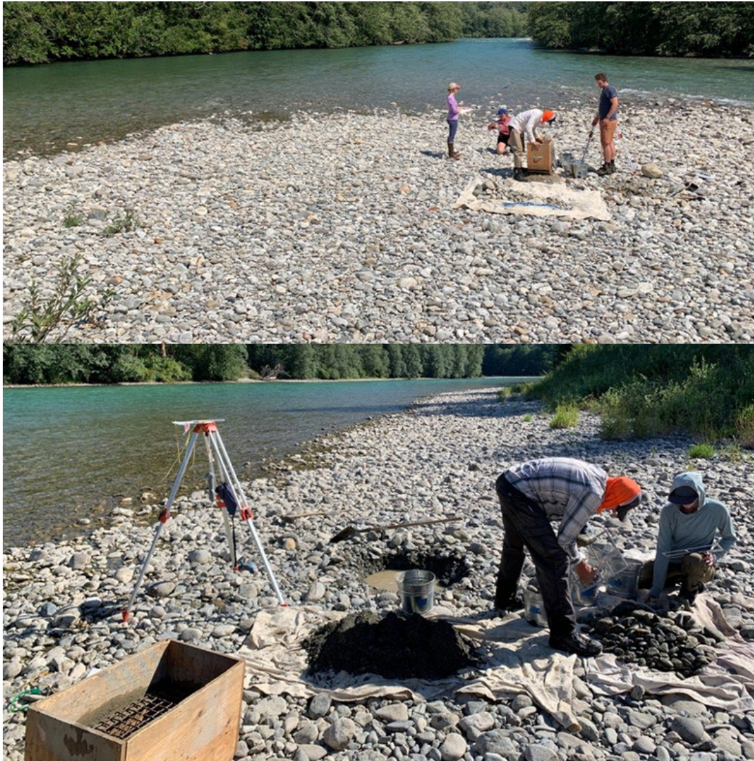
Figure 4.4-1. Examples of typical sediment sample locations, including the head of an island bar at PRM 90.2 (top) and head of a bank-attached point bar at PRM 78.4 (bottom).
