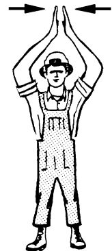
ALL OFF OR COMPLETED
