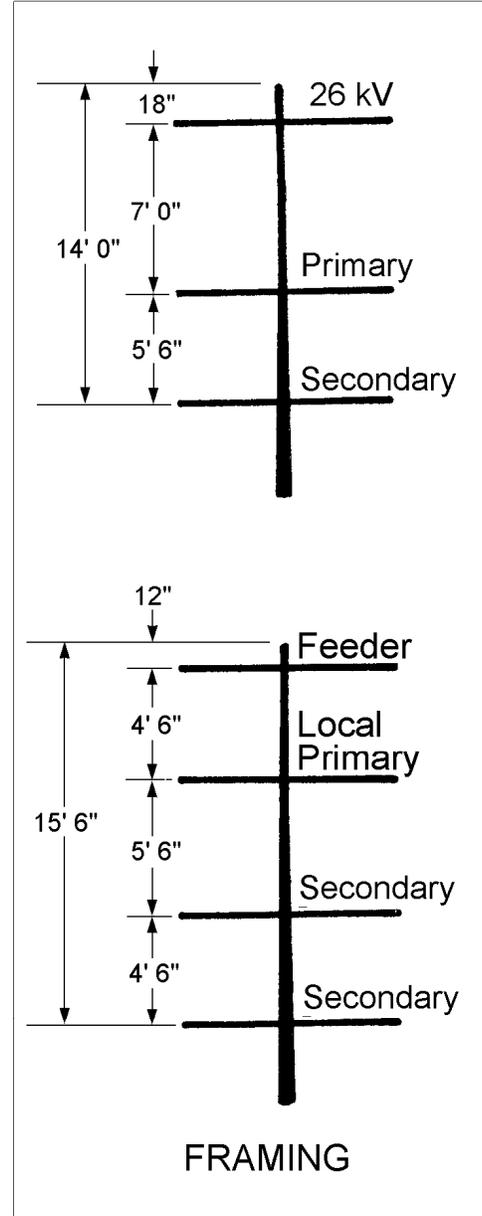
\*Increase 26kV arm spacing to 5 feet for 600 amp feeders within one mile of receiving substations and to 7 feet for 954 ACSR feeders (See D9-51.).
