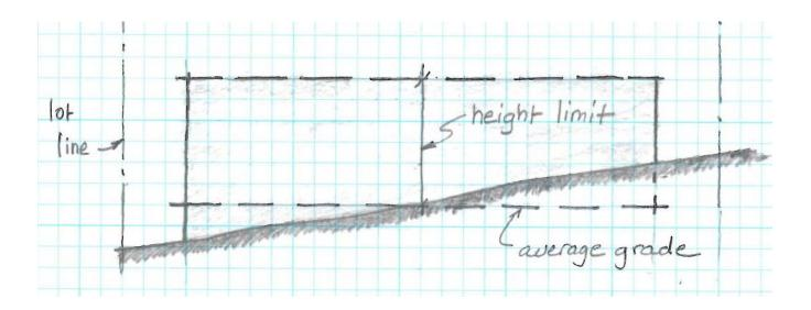
**Formula 1: Exterior Walls.** Under this formula, the average grade level is calculated as the average of the elevation of existing lot grades at the midpoints, measured horizontally, of each exterior wall of the structure enclosing occupied floor area.
