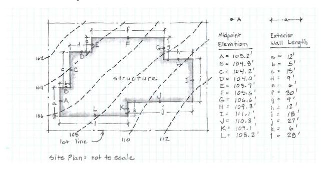
Formula:  $(A \times a)+(B \times b)+(C \times c)+(D \times d)+(E \times e)+(F \times f)+(G \times g)+(H \times h)+(J \times j)+(K \times k)+(L \times l)+...$ a+b+c+d+e+f+g+h+i+j+k+l+...
