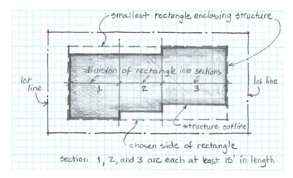
The average grade level for each section of the structure is calculated as the average elevation of existing lot grades at the midpoints of the two opposing sides of each section of the rectangle enclosing the structure, as shown below:
