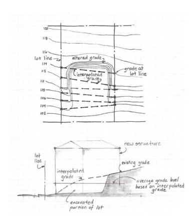
After the lot is developed, the grade must be restored from the lot lines used to establish the interpolated grade to the exterior walls of the building(s), following the general slope of the interpolated grade.
