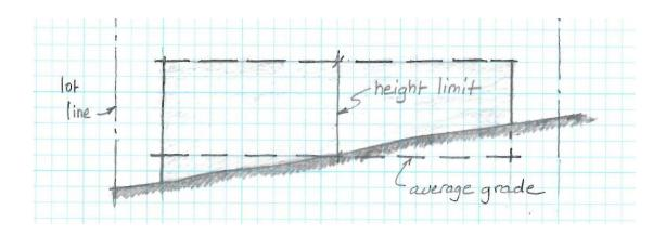
**Formula 1: Exterior Walls.** Under this formula, the average grade level is calculated as the average of the elevation of existing lot grades at the midpoints, measured horizontally, of each exterior wall of the structure enclosing occupied floor area.
