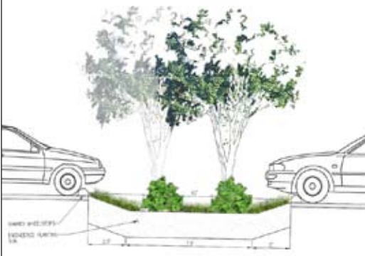
A telescoping swale optimizes performance by allowing for a wider vegetated swale between compact car parking stalls and narrower swales between standard size parking stalls.
