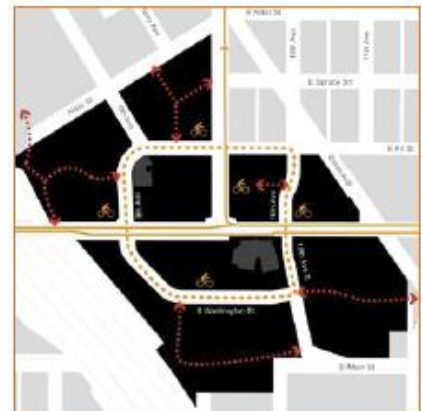
Conceptual bicycle circulation diagram Primary bike routes served by bike lanes, buffered bike lanes and sharrows are indicated with a solid orange line. The green street loop will provide secondary routes, as indicated with the dashed orange line. Access drives will provide through-block bike routes where topography allows; likely locations are shown with red dashed lines.
