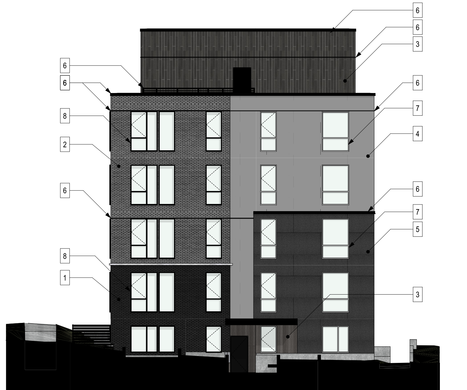
4 WEST RENDERED ELEVATION SCALE: 3/32" = 1'-0"
