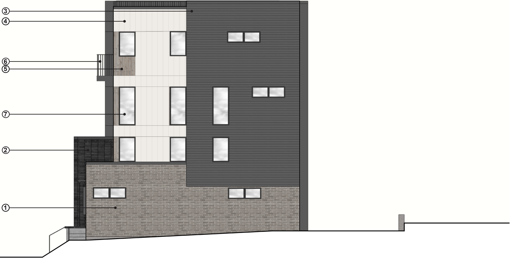
③ HORIZONTAL LAP SIDING SMOOTH W/ 5" EXPOSURE / FIBER CEMENT PANEL SW 7674 PEPPERCORN
