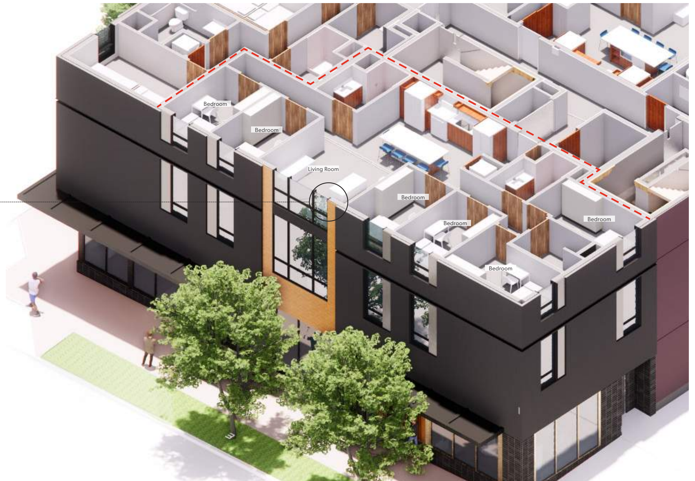
Section perspective view along 50th street, showing relationship of interior unit layout with exterior facade and window application.
