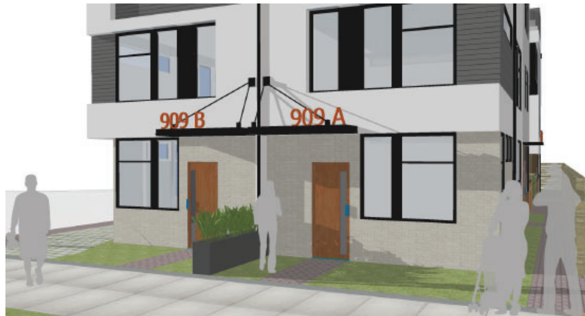
① Street level facade rendering / propose to use brick veneer facade in relation to the existing structure and modern form to accomodate the thriving new development along the NW 56th Street
