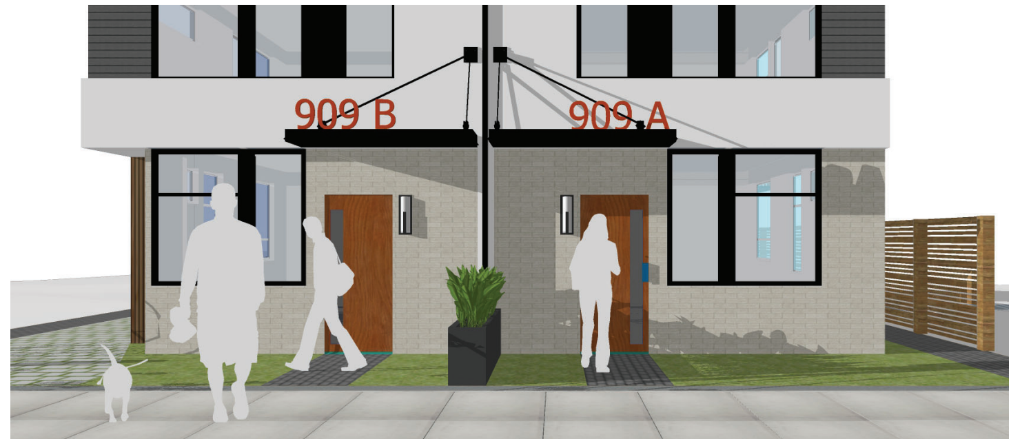
② Street level facade rendering / propose to use brick veneer facade
