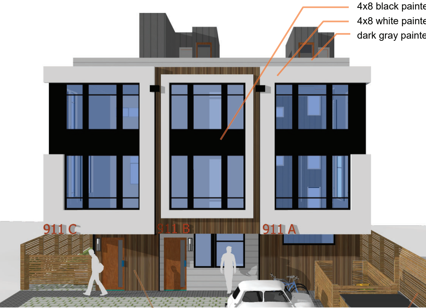
Townhouse 2 North Elevation Reclaimed vertical cedar siding cedar fence / horizontal
