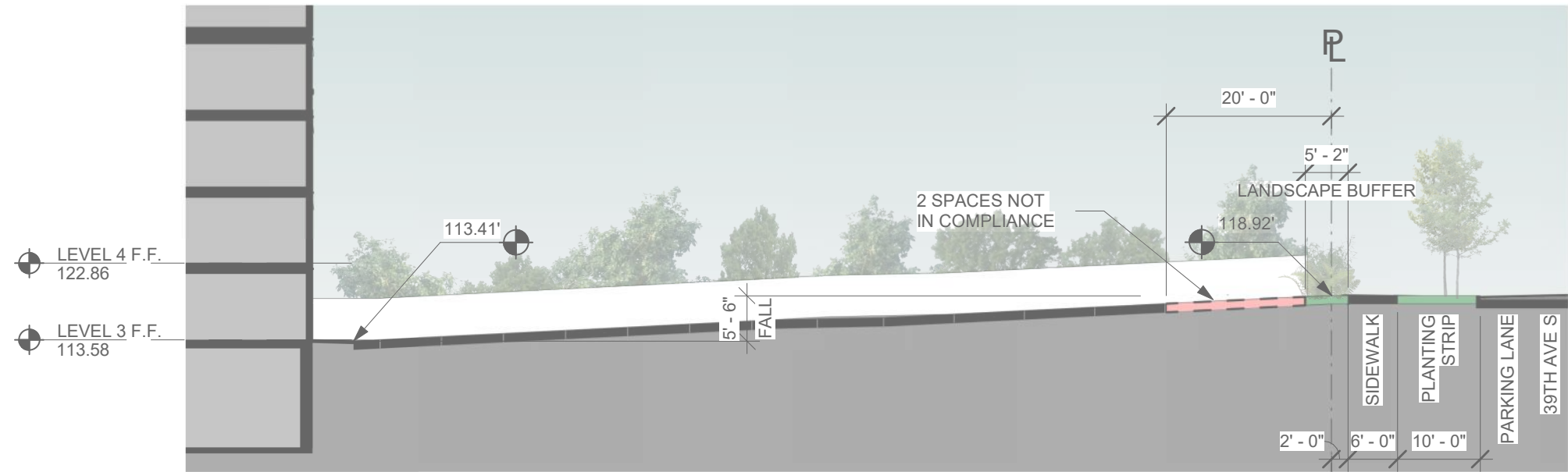
Figure 2: Site Section showing area of non-compliance, slope of the parking lot, layers of landscaping at the street frontage, and the site fence to the north of the parking lot.
