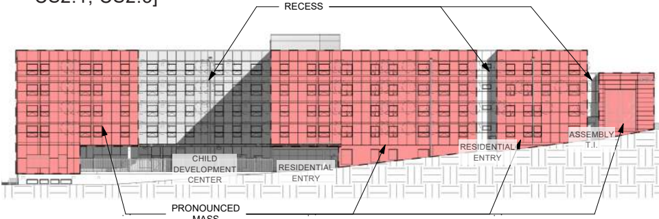
Figure CS1.1: Elevation showing how building responds to site elevation changes and locates pronounced masses and entries accordingly.
