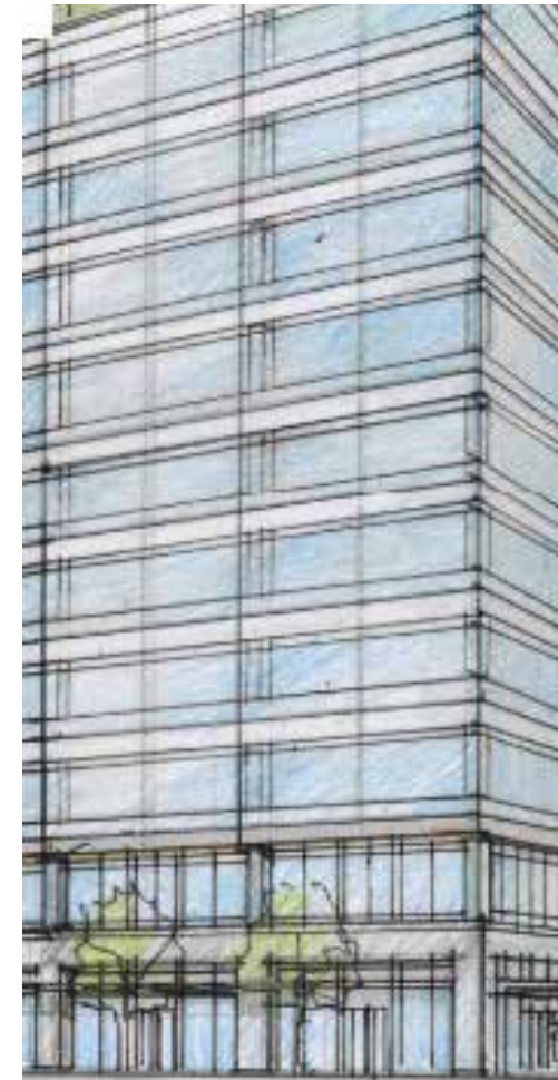
Facade study showing division of building into articulated base, recessed second floor and upper store curtainwall expression
