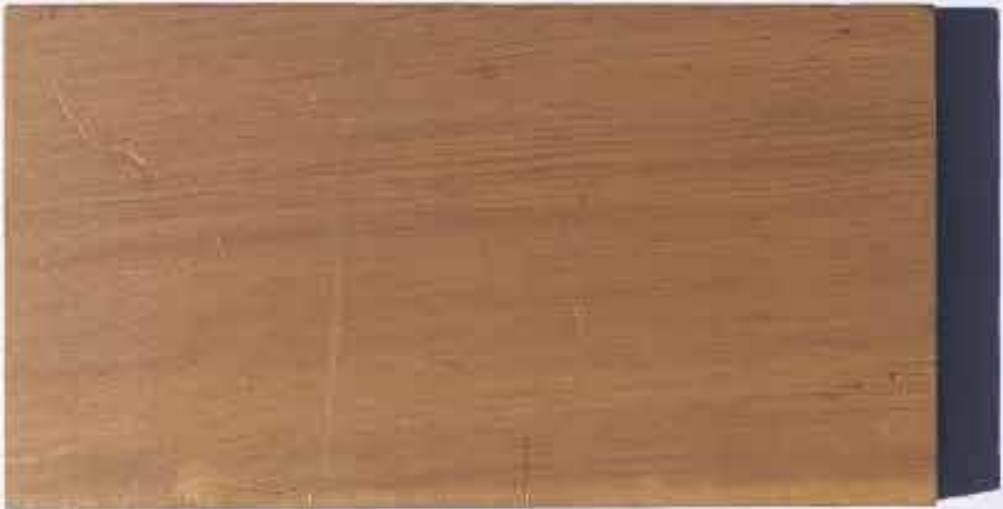
ACCENT SIDING + SOFFITS 1x4 T&G Cedar, Clear Coat Locations: Terrace units along Willow Street, back of exterior stair, roof deck; exterior soffits; underside of canopy at roof deck.
