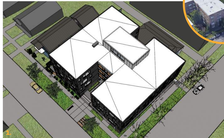
The symmetrical H shape splits the building in two bars to reduce perceived bulk on 15th Ave, which is a residential street, reserving the longer elevation for Jefferson, the arterial.
