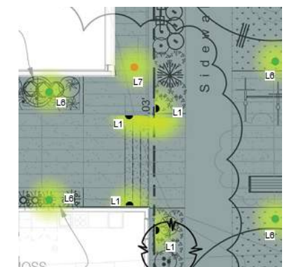
tread lights at courtyard
