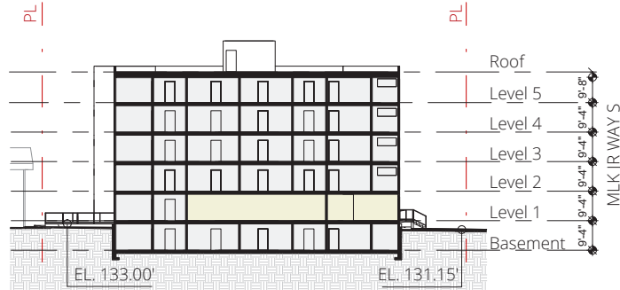
Section: Scheme A - Code Compliant
