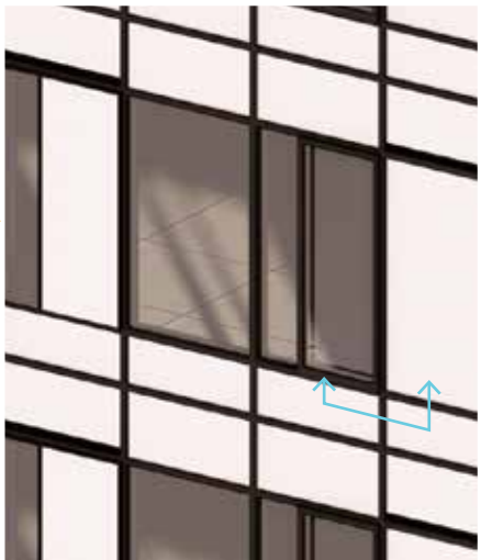
Flush Window Frame With Metal Panel
