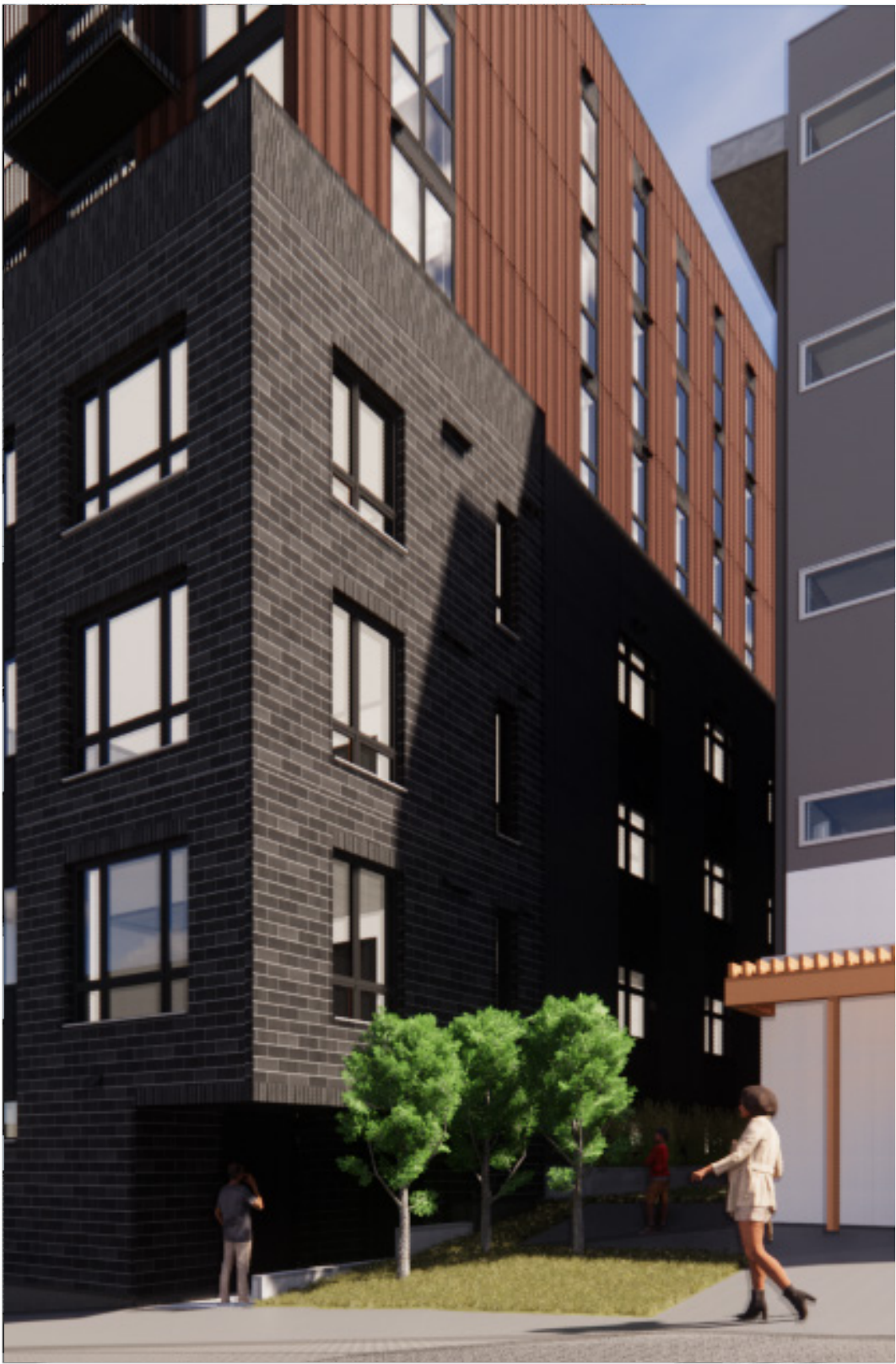
NORTHWEST ALLEY PERSPECTIVE ILLUSTRATING EXTENT OF BRICK MATERIAL
