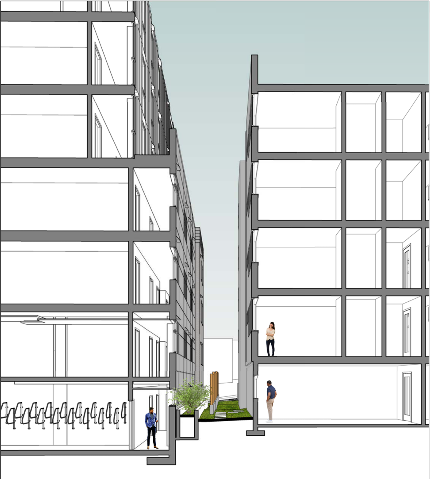
PARTIAL PERSPECTIVE SECTION SHOWING PASSAGEWAY BETWEEN LITTLEFIELD ANNEX AND SOL STUDIOS
