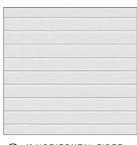
7 4" HORIZONTAL FIBER CEMENT LAP SIDING
