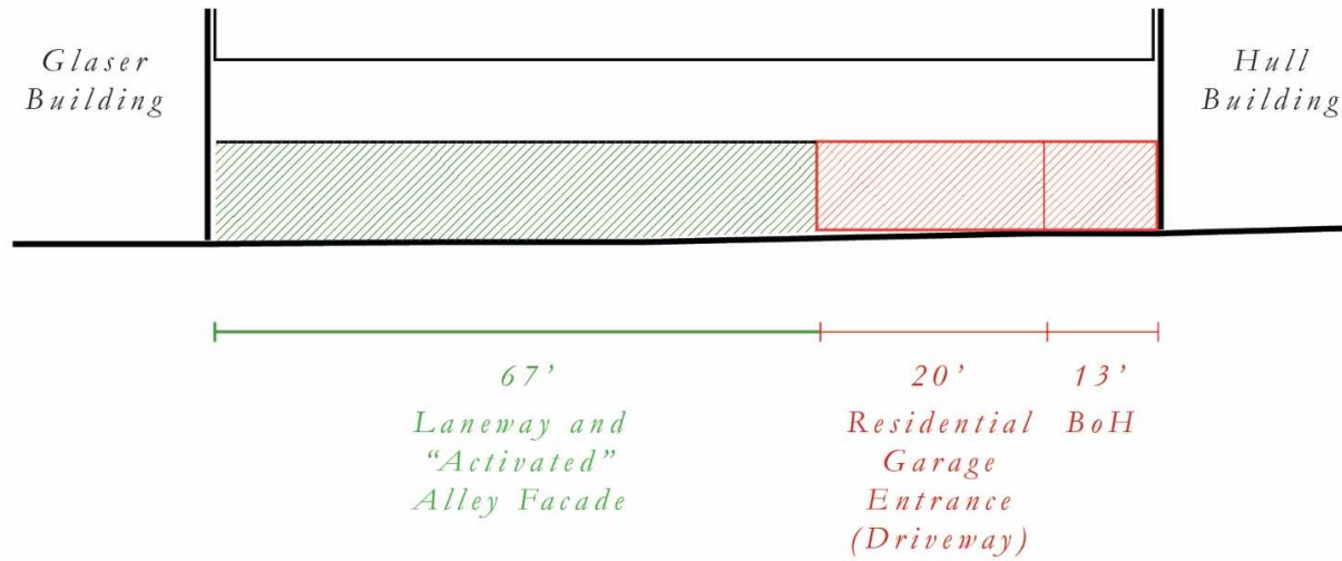
TWO-WAY TRAFFIC 20' WIDE DRIVEWAY (REQUIREMENT)
