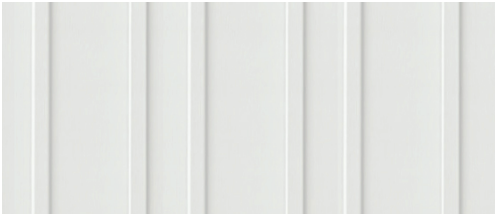
② FIBER CEMENT SIDING - WHITE PANEL THICKNESS: 5/16" - SMOOTH PATTERN: BOARD AND BATTEN BATTENS: 2-1/2" WIDE X 3/4" THICK PAINT FINISH: SW ICE CUBE MANUFACTURER: ALLURA, OR EQUIVALENT
