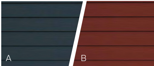
③ ACCENT FIBER CEMENT SIDING PANEL THICKNESS: 5/16" - SMOOTH PATTERN: LAP - 5 1/4" EXPOSURE COLOR: SW GALE FORCE (A) OR SW FIREWEED (B) MANUFACTURER: ALLURA, OR EQUIVALENT
