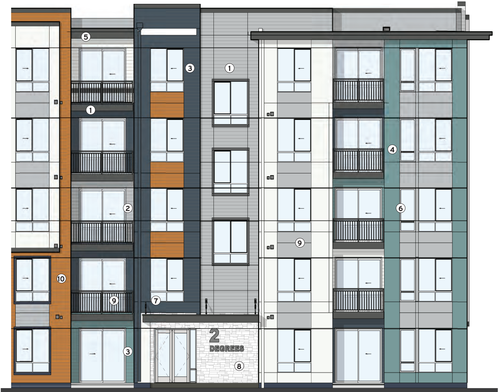
② FIBER CEMENT LAP SIDING PANEL THICKNESS: 5/16" - SMOOTH PATTERN: LAP - 5 1/4" EXPOSURE COLOR: SW LAZY GRAY OR SW HIGHLY REFLECTIVE WHITE MANUFACTURER: ALLURA, OR EQUIVALENT
