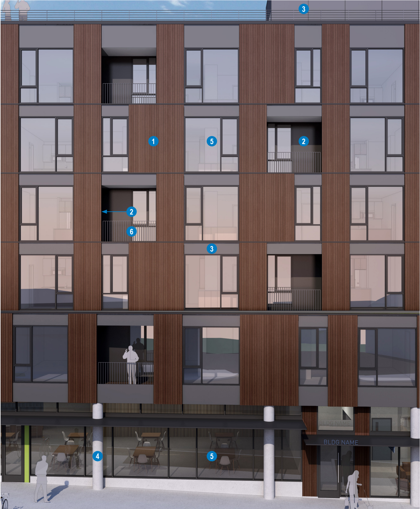
2 METAL PANEL 1 // CHARCOAL 5' X 20' ACM PANEL, 1/8" THICK
