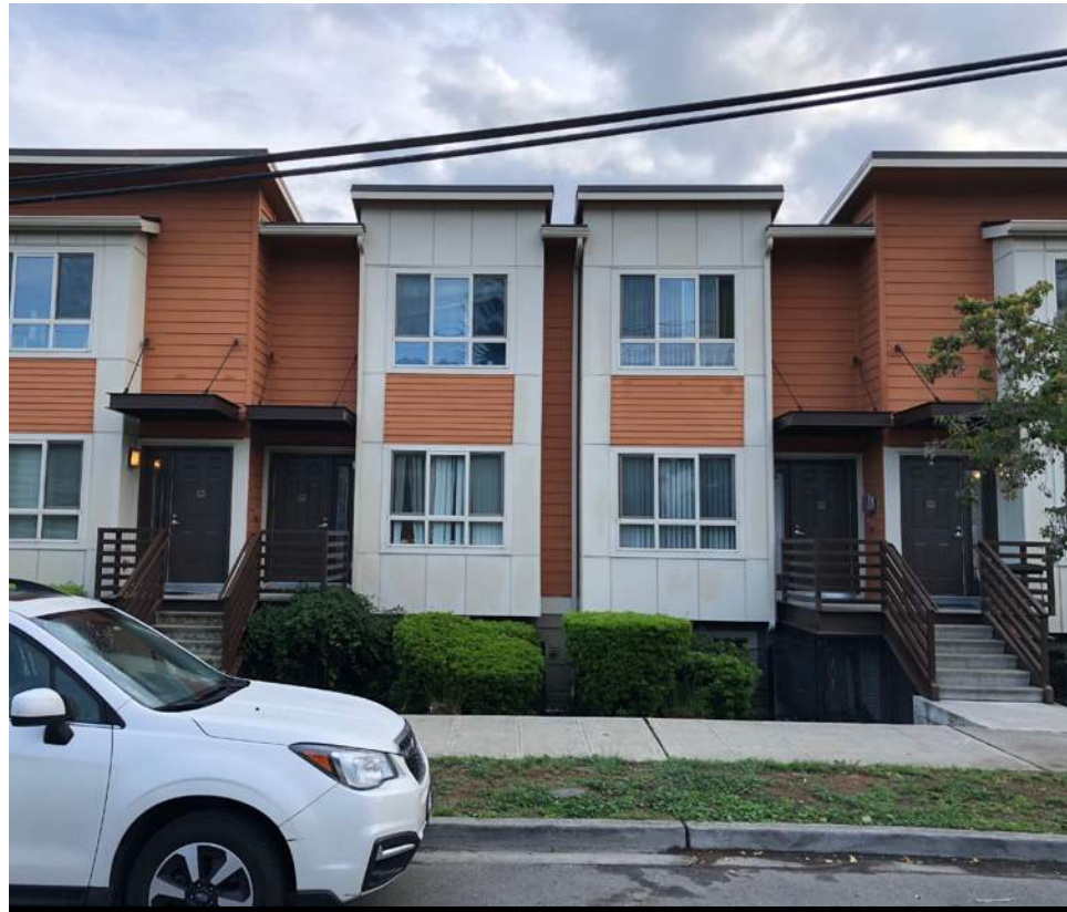
Design Cues: Elevated First Floor, Eyes on the Street, Articulated Building Mass
