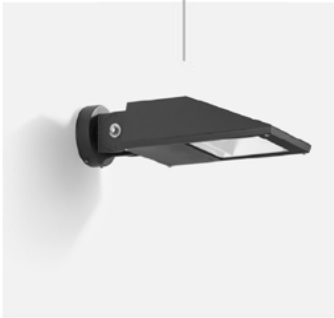
L4 Wall-pack with cut-off optics and forward light distribution, also serving egress illumination. 4000 K CCT
