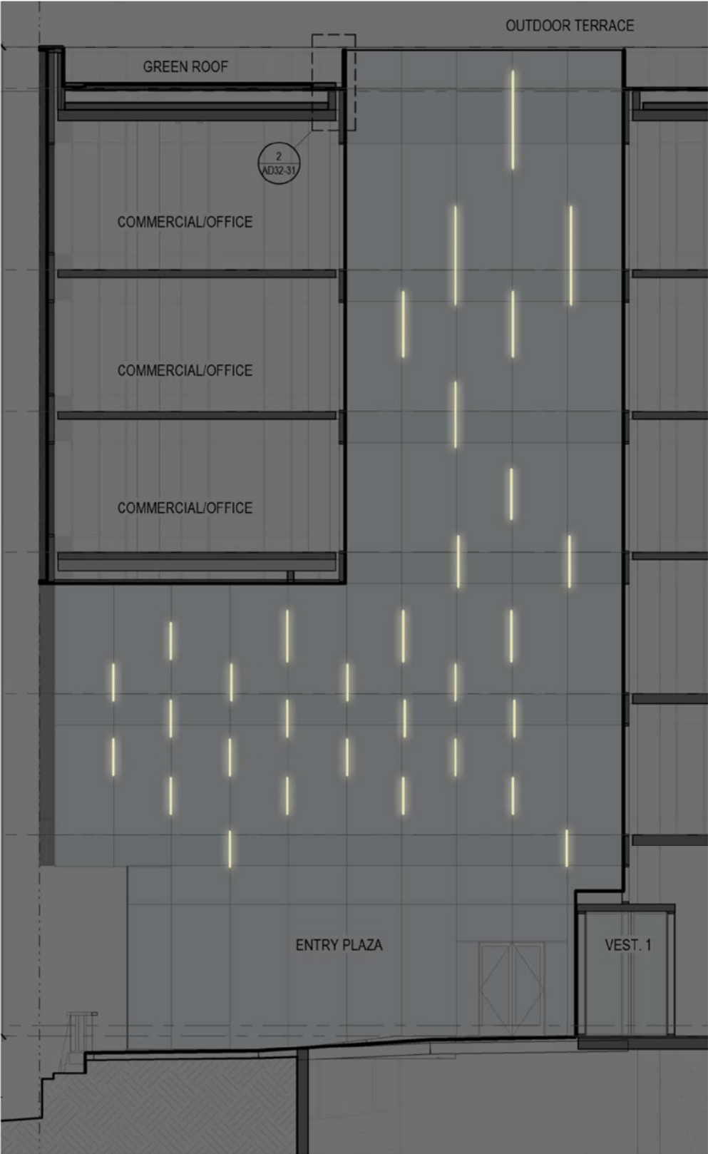
L1 Thin LED profile with direct-view optics. Art installation Integrated with the mullion system. 3000 K CCT
