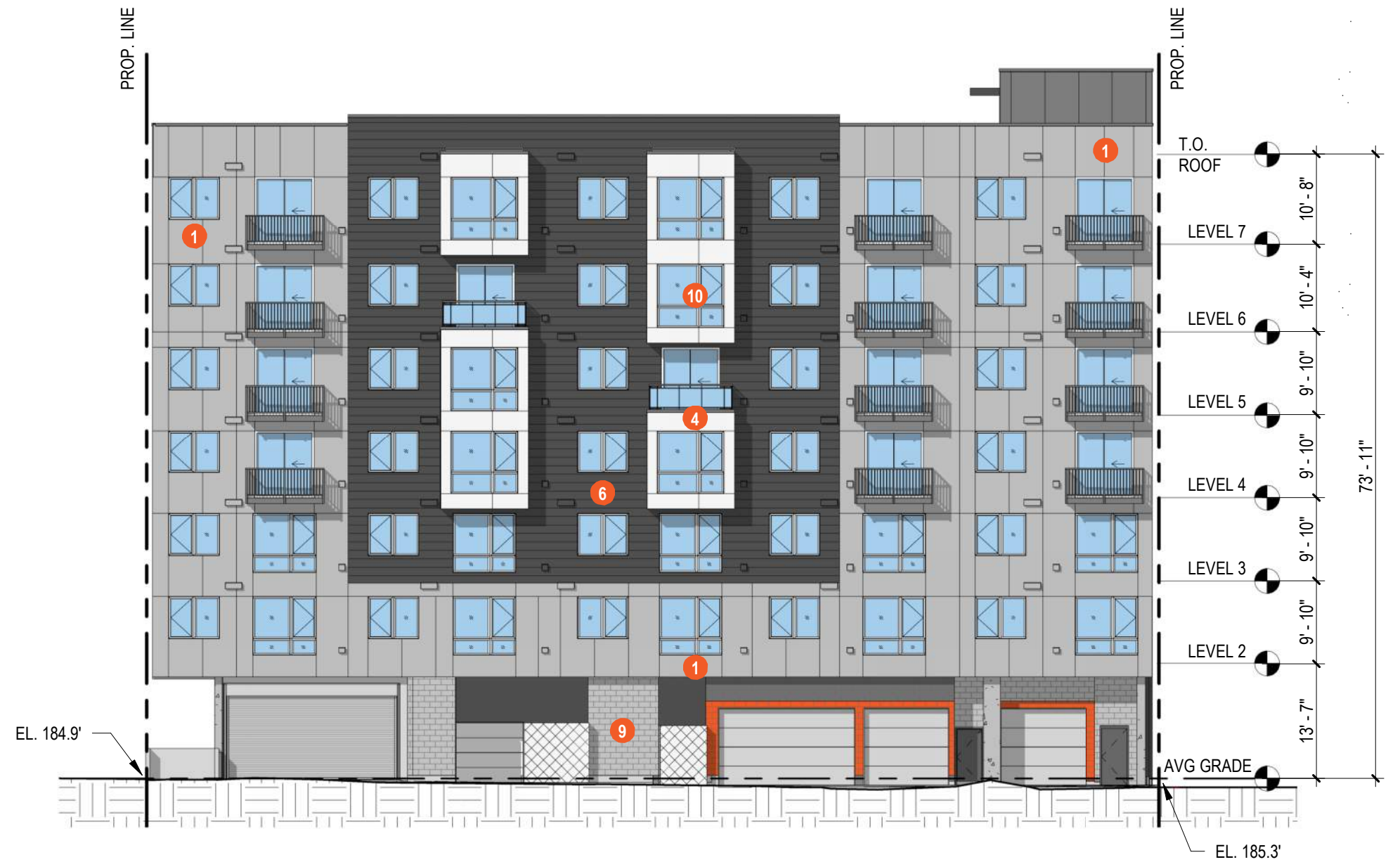
WEST ELEVATION - ALLEY 1/16" = 1'-0"
