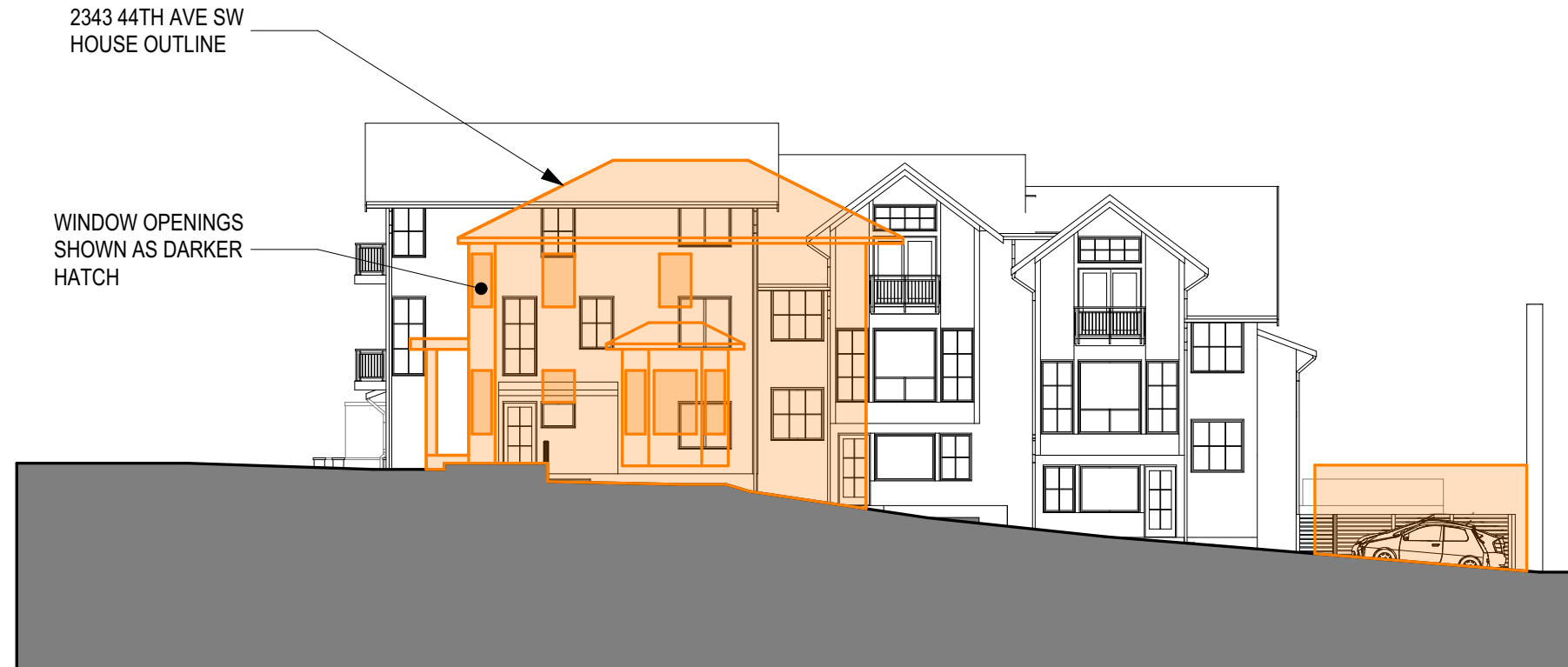
NORTH ELEVATION - WINDOW ADJACENCY
