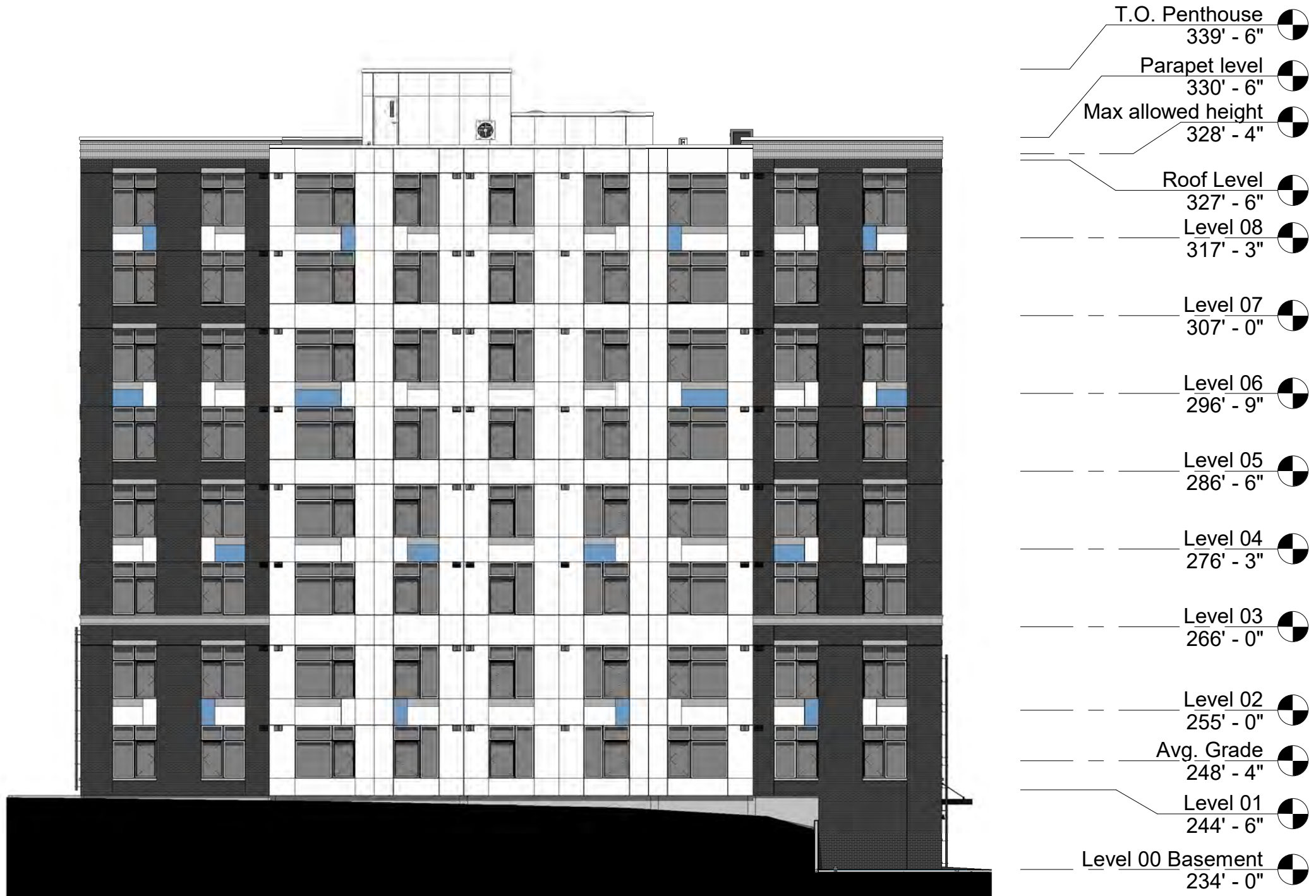
① Elevation North 1/16" = 1'-0"
