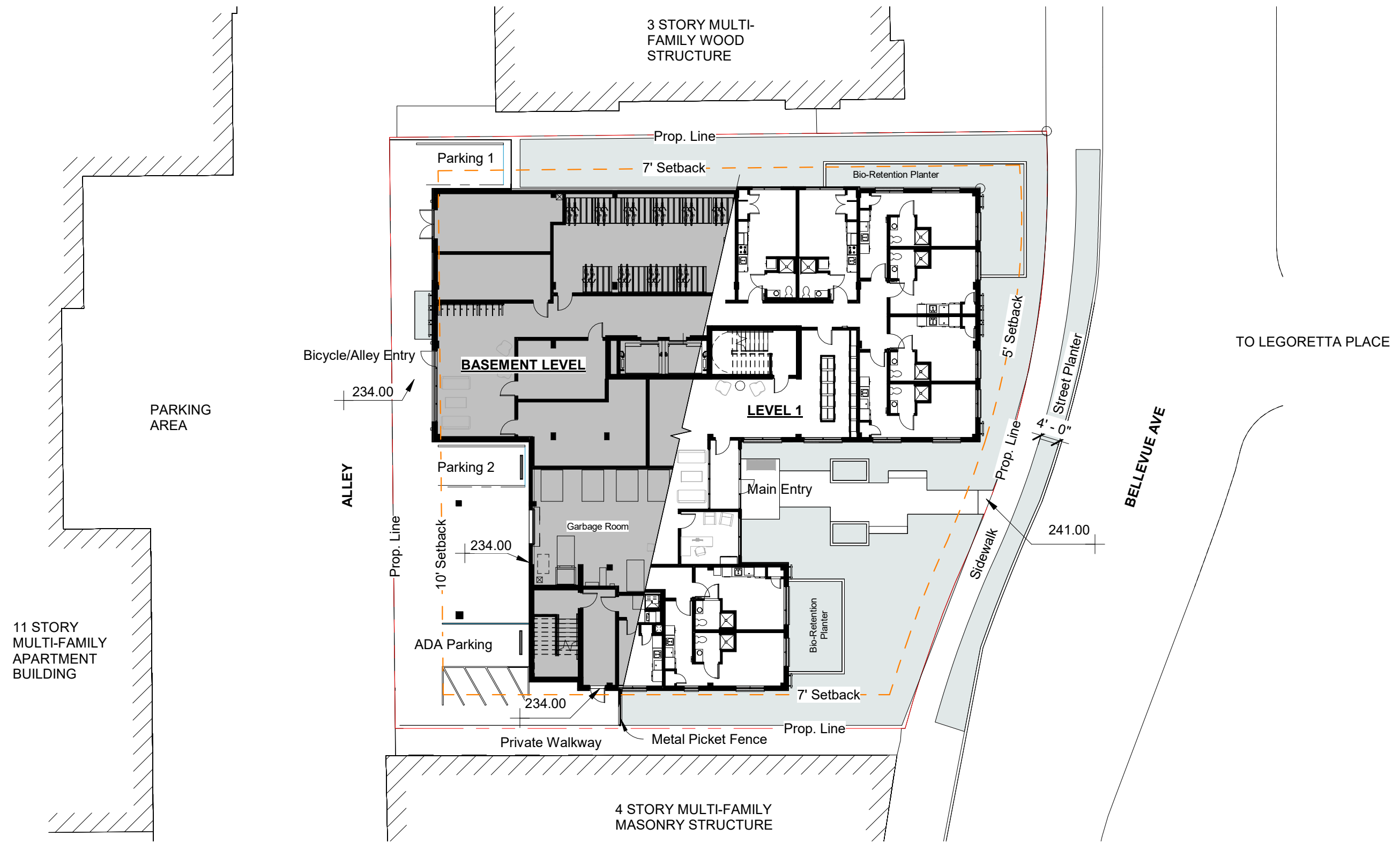
① BASEMENT/LEVEL 01-SITE PLAN 3/64" = 1'-0"
