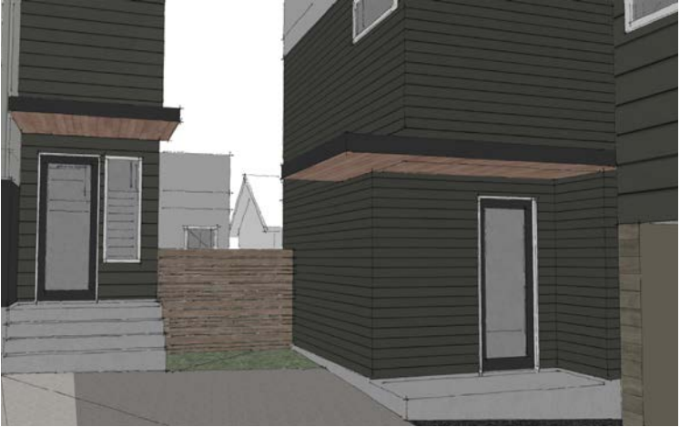
Use of cedar siding at entries, along the pedestrian walkways and at yard areas provides a fine-grained texture and warmth that relate to the human scale & helps to identify entries.
