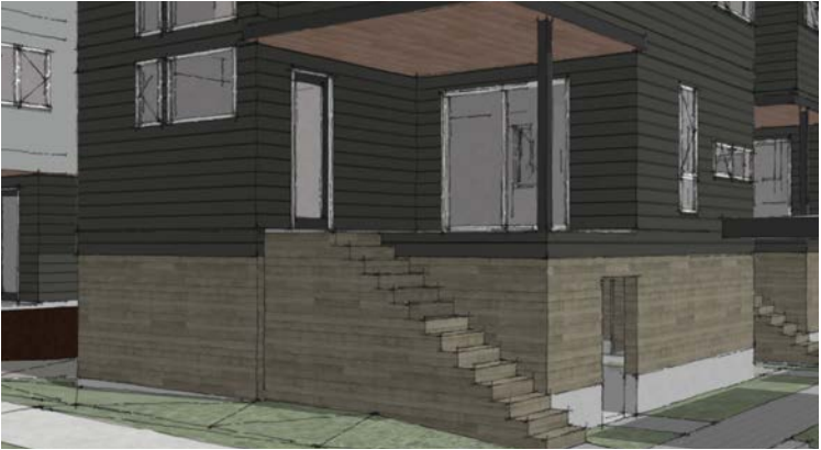
Cedar siding provides texture & pattern at the pedestrian level in an area that would otherwise be a blank facade.
