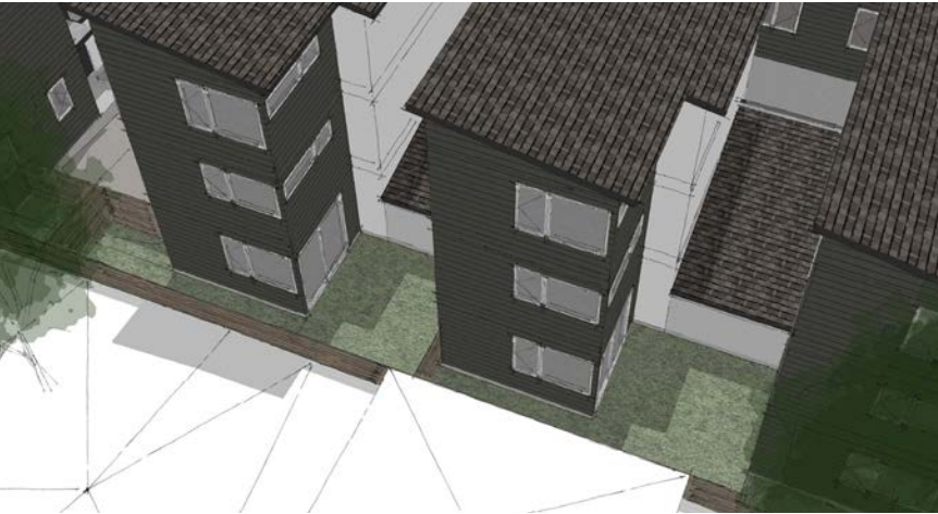
Units 1-3 have primarily north facing yards so the building massing steps down between units to allow more sunlight to reach the yard area.
