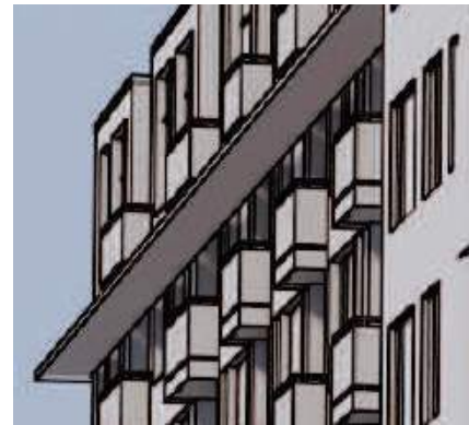
A horizontal brise soleil at the next-to-top floor reduces the perception of the top floor from a street level aspect.
