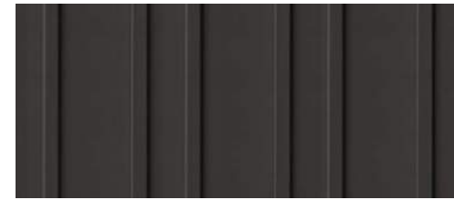
② FIBER CEMENT SIDING PANEL THICKNESS: 5/16" PATTERN: BOARD AND BATTEN BATTENS: 2-1/2" WIDE X 3/4" THICK PAINT FINISH: DARK GRAY
