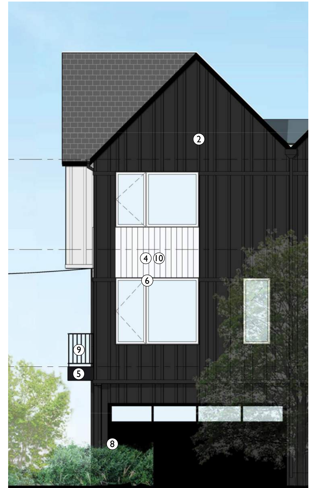
④ METAL ACCENT PANEL PANEL GAUGE: 24 PROFILE: BOX RIB POWDER COAT FINISH: BLACK OR WHITE
