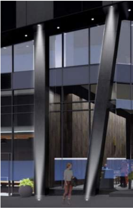
SOFFIT MOUNTED GENERAL/COLUMN DOWNLIGHTS + IN-GRADE COLUMN UPLIGHT
