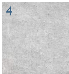
4 Architectural Concrete Natural Smooth-Form Finish
