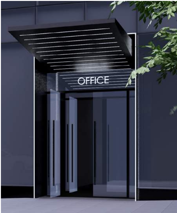
RECESSED LINEAR LENSED FIXTURE AT OFFICE AND RESTAURANT CANOPIES
