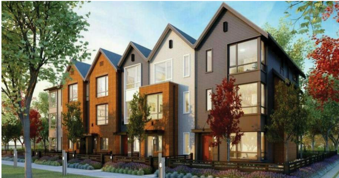
Modulation with articulated roof forms Restrained material palette Weather protection at entries
