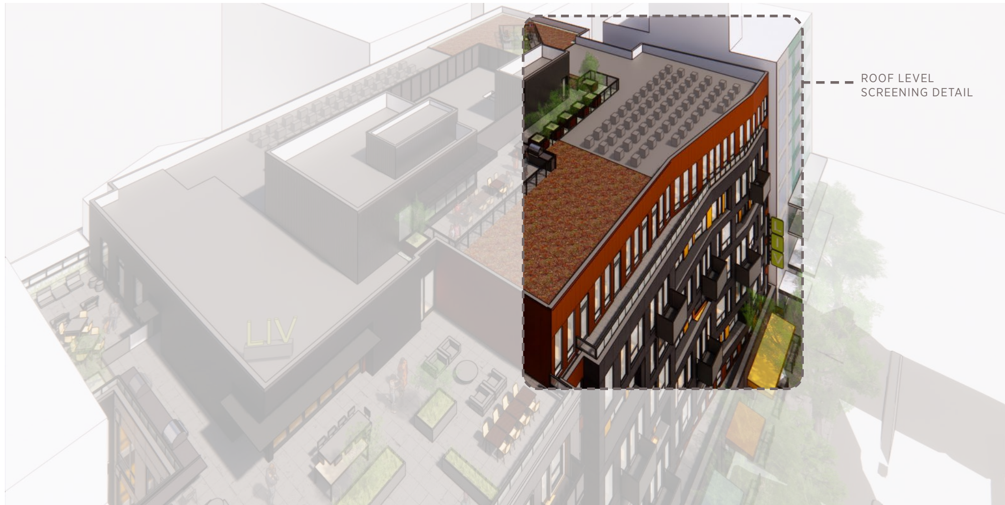
MECHANICAL SCREENING DIAGRAM: THE PARAPET HEIGHT ALONG 2ND AVE HAS BEEN REVISED TO THE MINIMUM NEEDED TO CONCEAL ROOFTOP COOLING EQUIPMENT. THE TAPERED PROFILE RECALLS THE ELEVATION OF THE ADJACENT STRUCTURE TO THE SOUTH WHILE NOT MATCHING IT.
