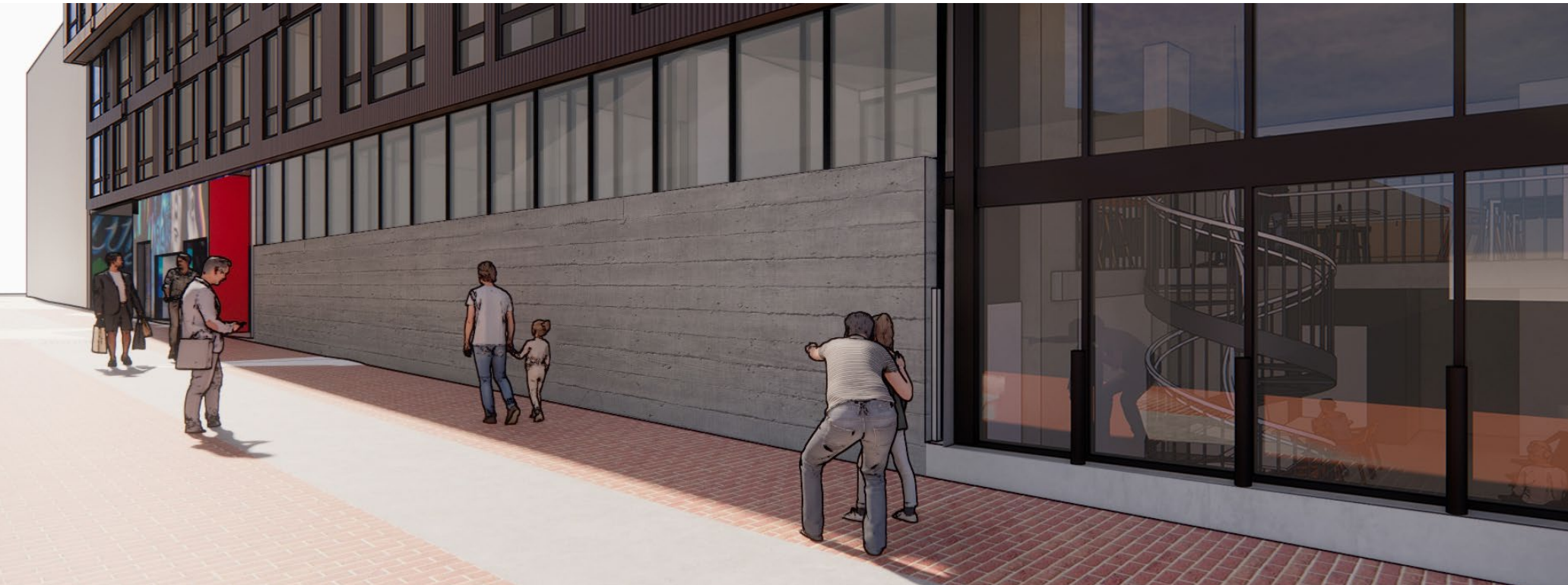
ALLEY VEHICLE BARRIER STUDY - TEXTURED BOARD FORMED CONCRETE
