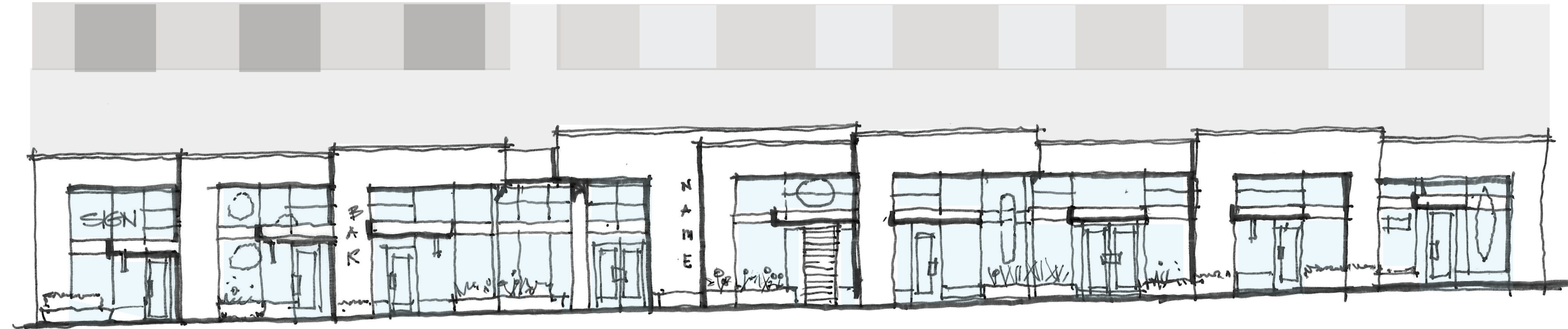
BASE OF BUILDING CHARACTER STUDY 3 - INDIVIDUAL TENANT SPACES ARE EXPRESSED IN VARIATION IN ARCHITECTURAL FORM RATHER THAN RELYING ON TENANT CUSTOMIZATION. THOUGH, THAT COULD BE ACCOMODATED AS WELL. THE MODULATION WIDTH FOLLOWS THE PATTERN OF EXISTING NARROW STOREFRONTS ALONG THIS STRETCH OF 2ND AVENUE.
