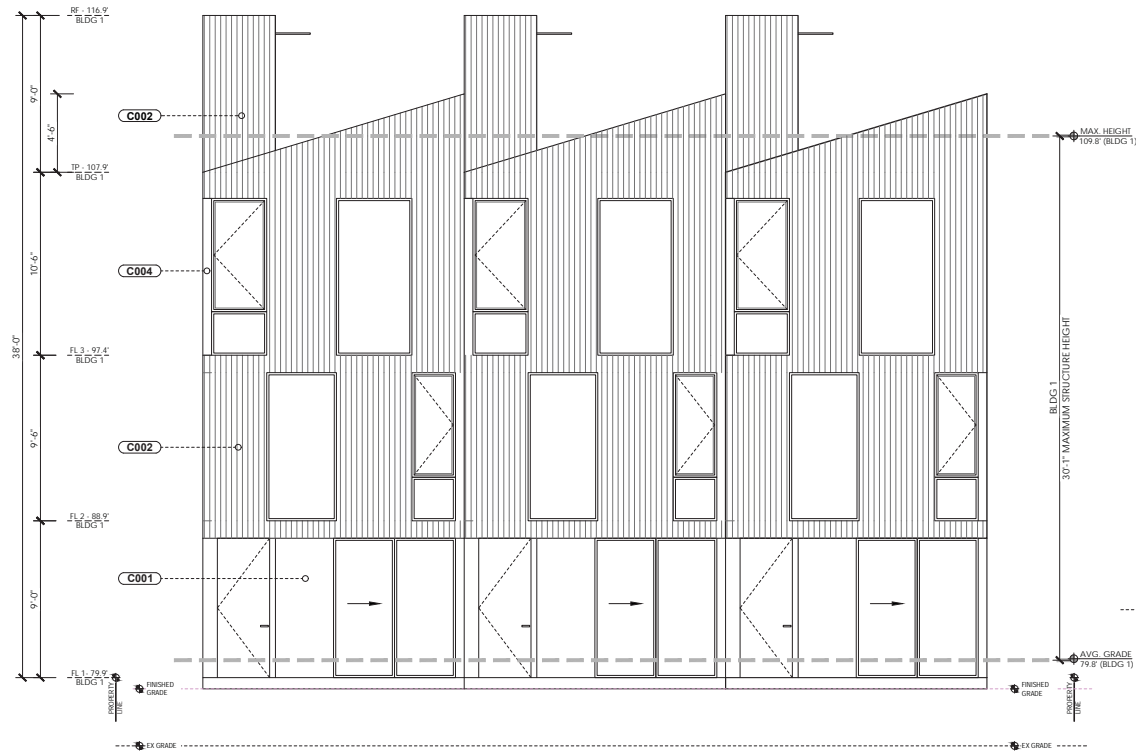
North Elevation BLDG 1 SCALE: 1/4" = 1'-0"
