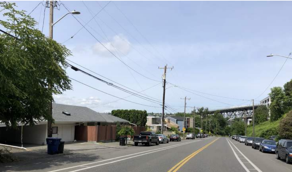
Power Lines on Dexter Ave N require 14' clearance per SCL
