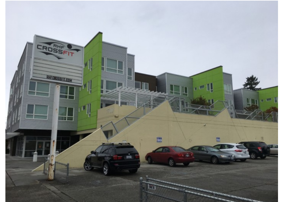
Emerald City Commons : Note façade modulation, roof lines, fiber cement cladding and simple geometry
