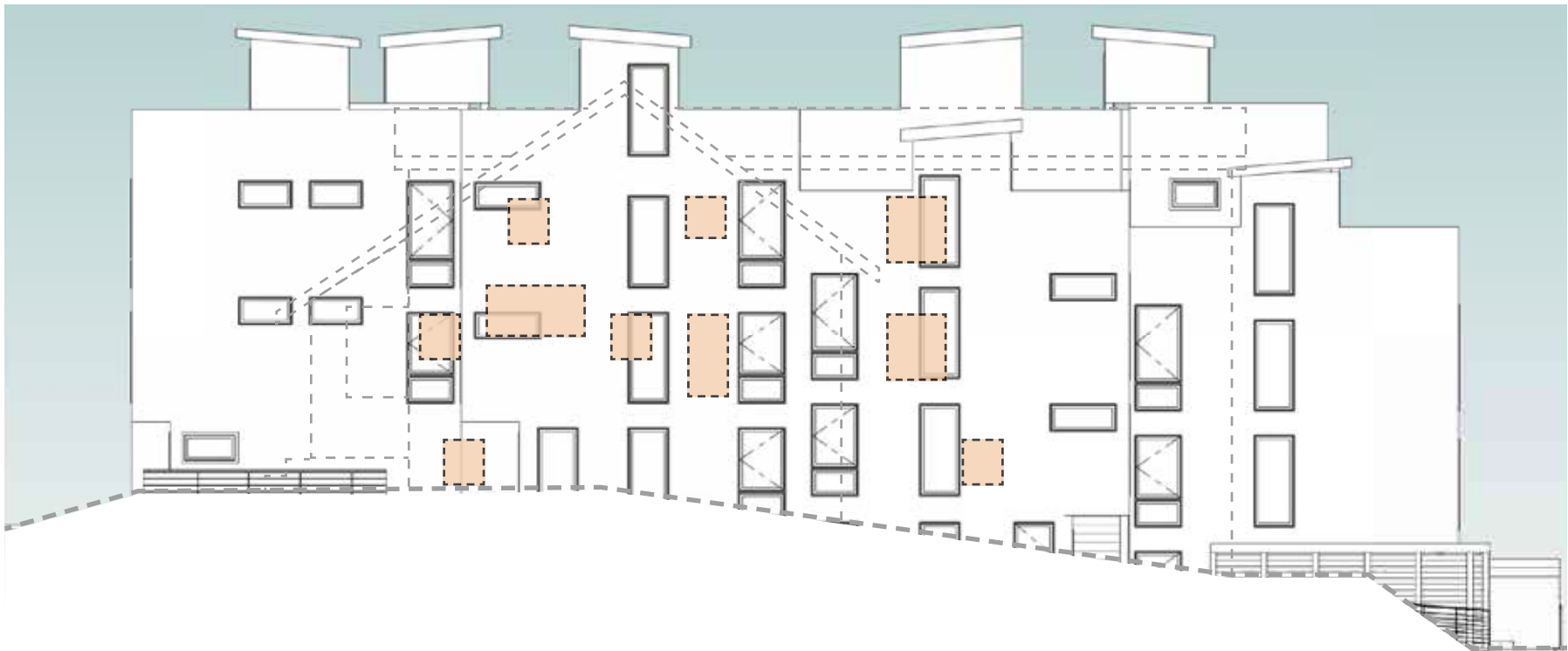
SOUTH ELEVATION: WINDOW LOCATION OVERLAY WITH ADJACENT STRUCTURE
