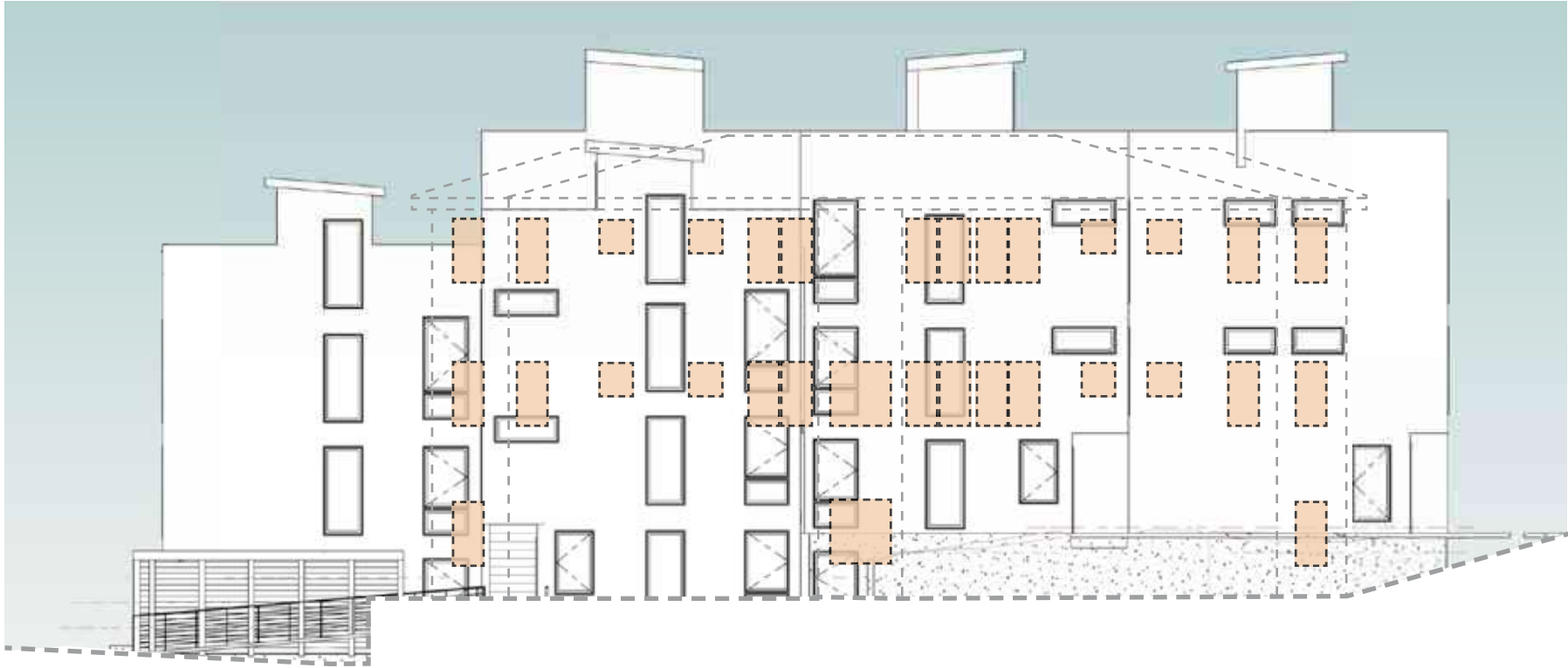
NORTH ELEVATION: WINDOW LOCATION OVERLAY WITH ADJACENT STRUCTURE
