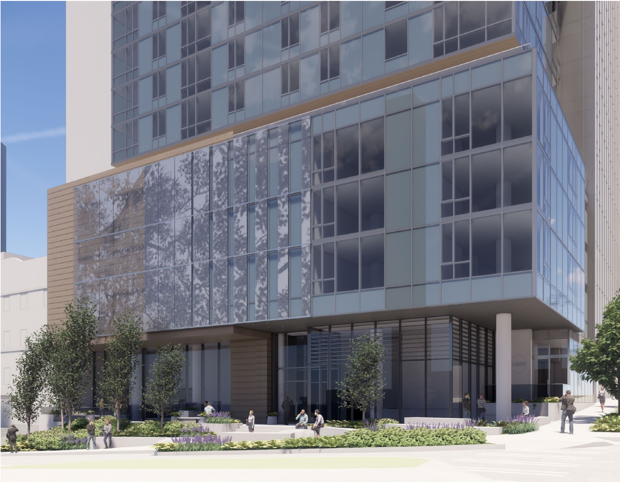
Initial concept for a metal screen option that could feature a canopy/vegetation pattern that conceptually continues the tree canopy up the facade, dissipating as it blends the solid and glass treatments together.
