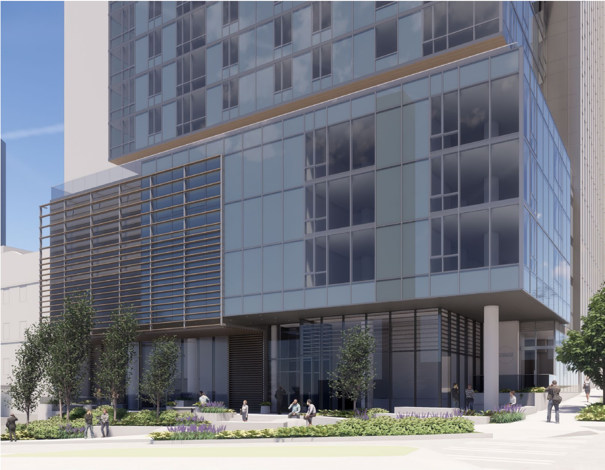
Initial conceptual study of a wood like metal slat option that would wrap up from the ground level, creating a soffit over the porch, and dissipating as it climbs the podium and reveals the tower forms and treatments.
