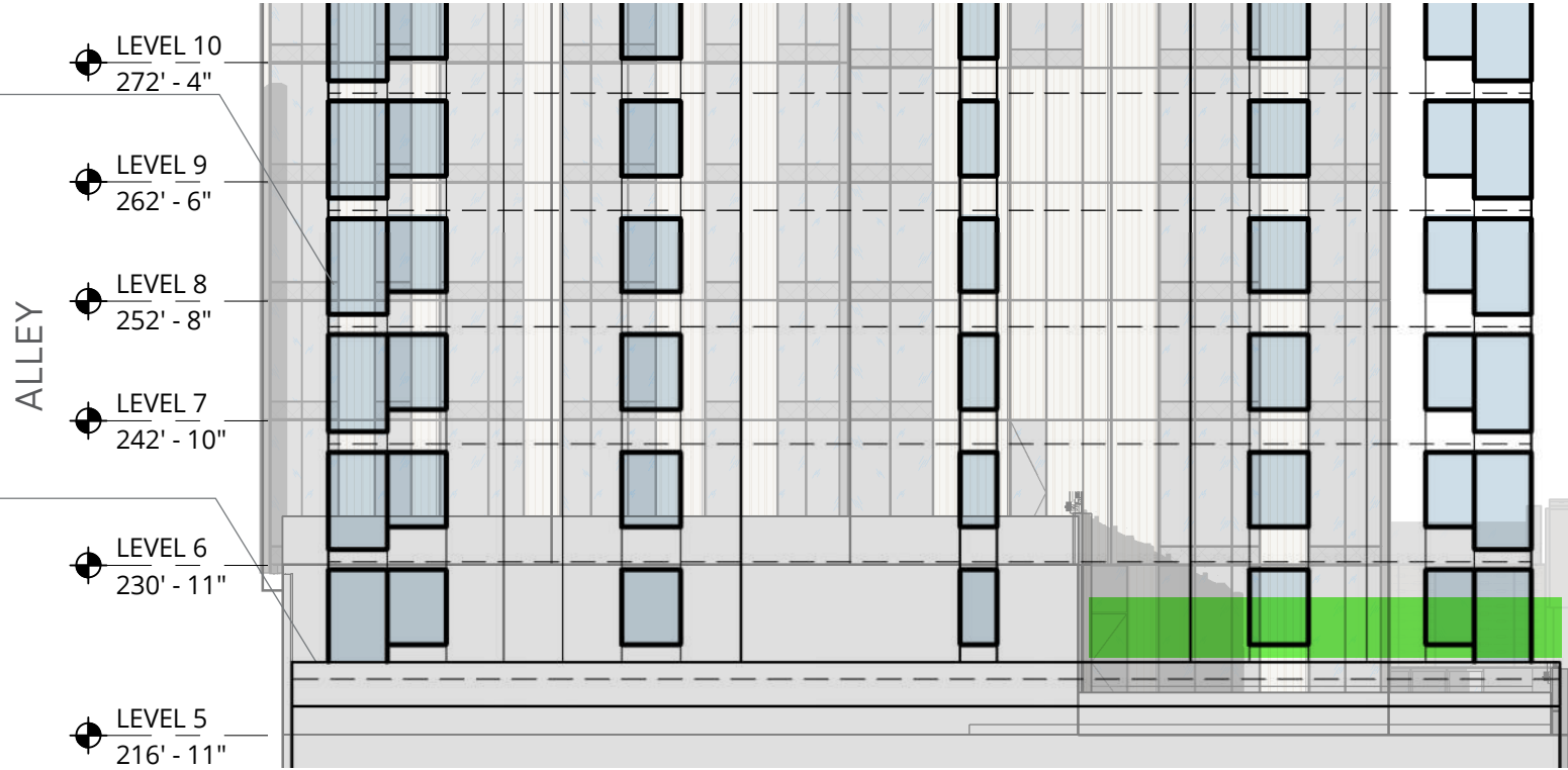
PARTIAL SOUTH ELEVATION - VIKTORIA WINDOW OVERLAY SCALE: 1/16" = 1'-0"
