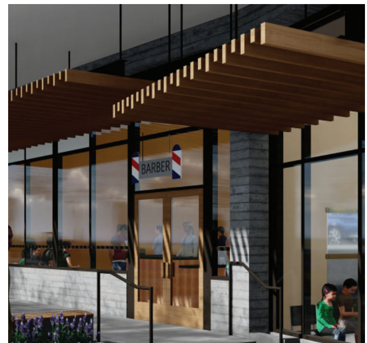
9 - TRELLIS - METAL FABRICATIONS MATCH NATURAL FIR COLOR
