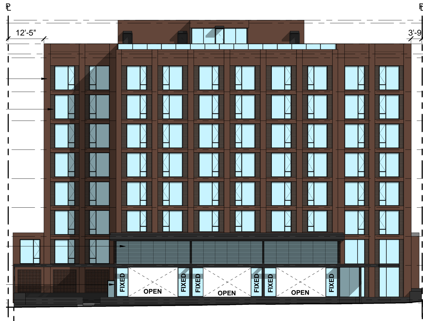
SOUTH ELEVATION - SLIDER WINDOWS AT STOREFRONT (OPEN)
