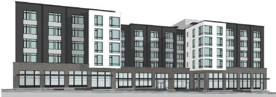
Proposed Design - The lanterns echo proportioning of the golden section while better matching the verticality established by adjacent facades. This design also provides more courtyard facing glazing - further reinforcing the importance of that space.
