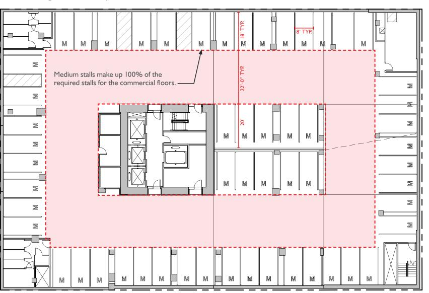
Commerical office stalls are located on the first two levels of the below grade parking, but the layout is identical to the floors below.
