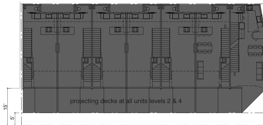
code compliant plan - projecting balconies
