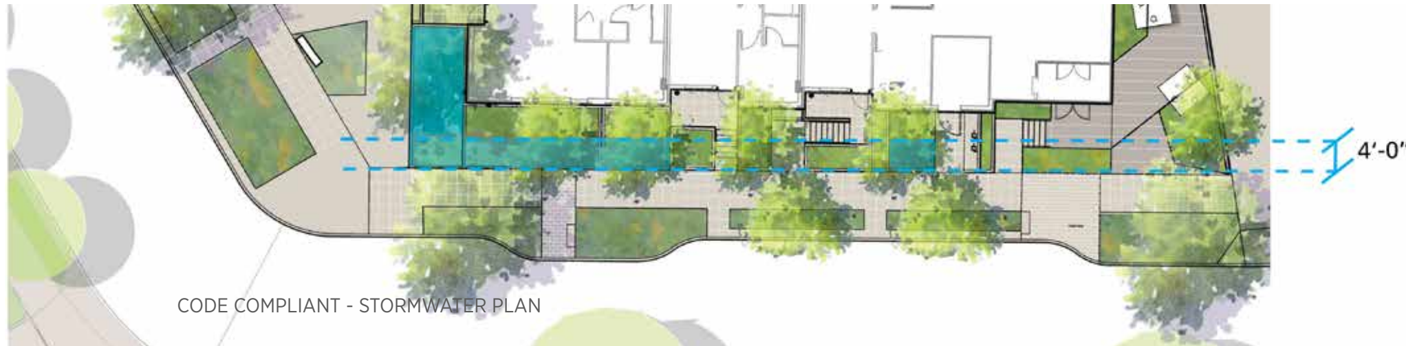
CODE COMPLIANT - STORMWATER PLAN
