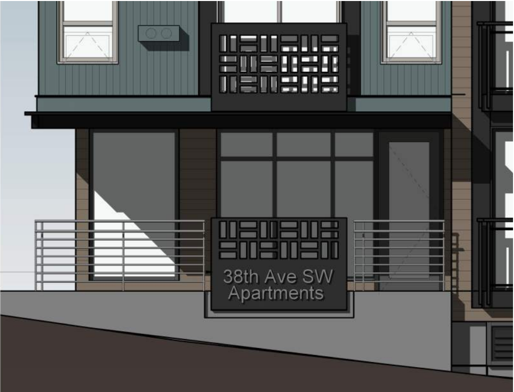
BUILDING SIGN LASER CUT BACK- LIT METAL, PAINTED DARK GRAY
