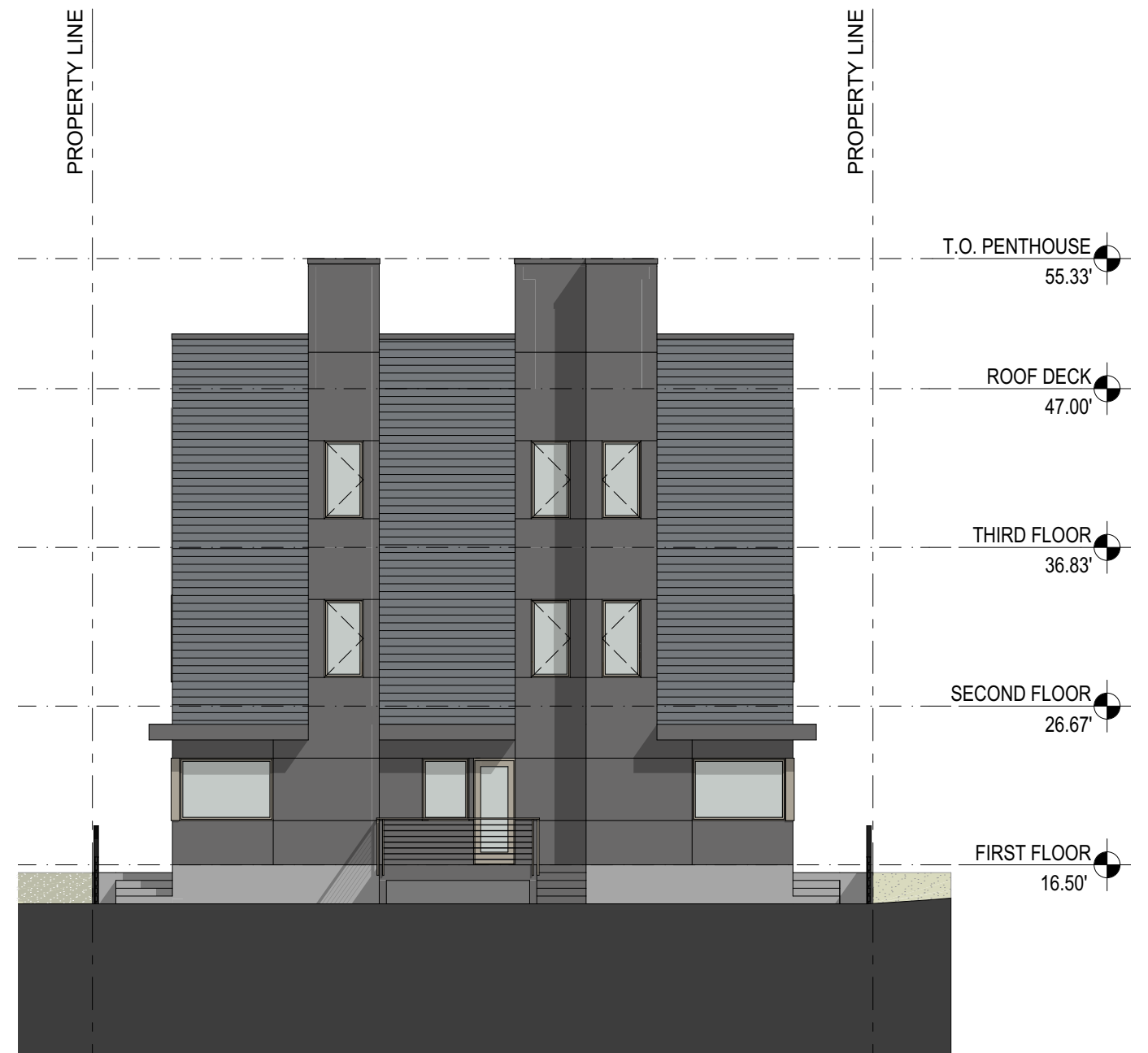
BUILDING 1. NORTH ELEVATION
