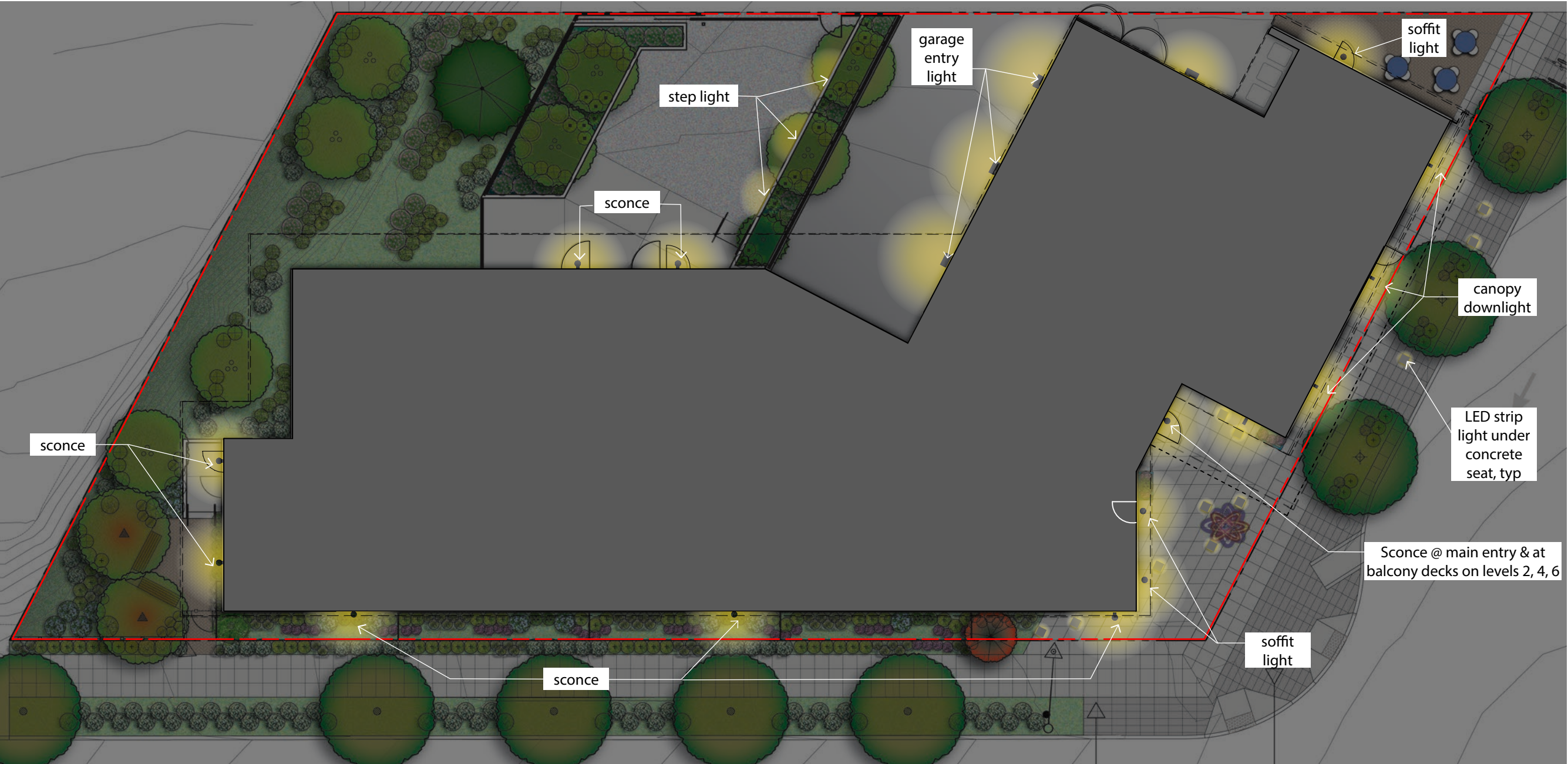
DOWN LIGHT SCONCE finish: brushed aluminum Wall-mounted down lights are located on the concrete piers along Rainier Ave., at the South open space, Main Entry, and Loading area.
